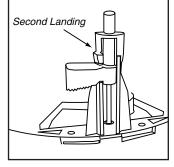
than 54 mm (2.125 inches) thick, start with the dog ear in the second (top) landing to ensure clearance and ease of installation.
